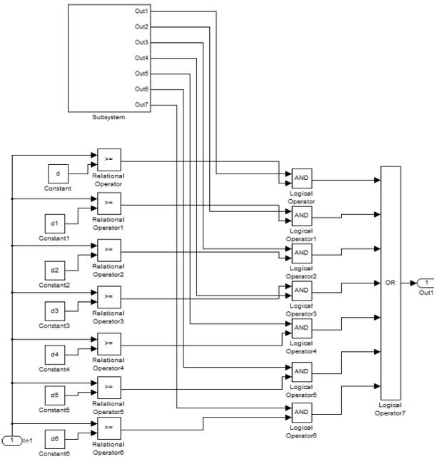
Fig. 7. Control circuit of the charging posts.
