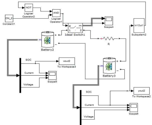
Fig. 8. System for controlling the charging process of the EV battery.
