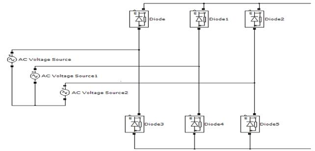
Fig. 5. Three-phase bridge rectifier.
