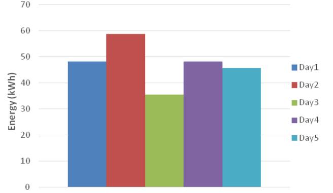
Fig. 10. Total energy provided by the charging posts each day (initial simulation).
