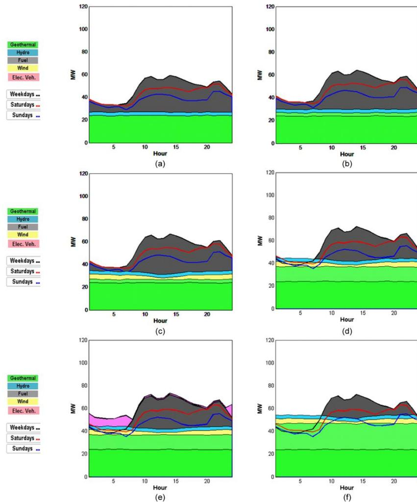
**Fig. 5.** Spring electricity load profile: a) Base year (2007), b) Addition of 3 MW geothermal (2010), c) Addition of 9 MW wind (2011), d) Addition of 10 MW geothermal (2011), e) Addition of 32% EVs (2013), and f) Addition of 10 MW geothermal without EVs (2013). Cases b to f are accompanied by a 4% increase of electricity demand
