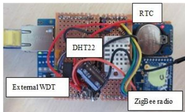
Figure 9: Coordinator photograph. An external Watch Dog Timer (WDT) circuit has been added to allow for reset of the microcontroller in case of malfunction. The Real Time clock, the Zigbee radio and the DHT22 sensors are clearly visible in the image [20].
