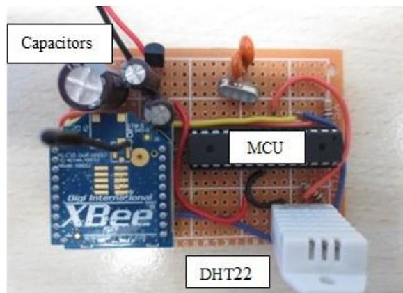
Figure 8: Photograph of sensor node built on stripboard. The MCU, the sensor and other electronics components can be appreciated in the picture [20]
