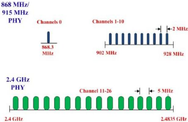
Figure 4: ZigBee channel allocation by [18]
