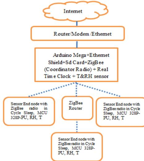
Figure 7: Sketch of the wireless sensor network connected to the internet [20]
