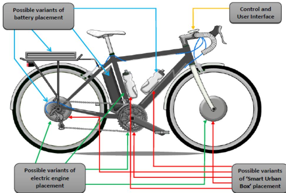
Figure 5: Sketch of the proposed design electric vehicle with its installed ‘Smart Urban Box’
