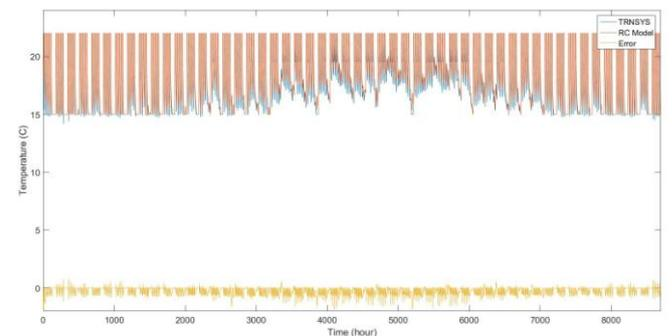
Fig. 9. Temperature for RC model comparing to TRNSYS for one year
