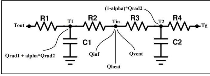
Fig. 1. 4R2C model for making the simplified building model
