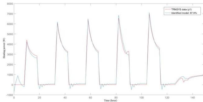
Fig. 2. 150-hour time response comparison for heating load
