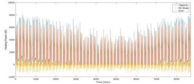
Fig. 8. Heating load for RC model comparing to TRNSYS for one year
