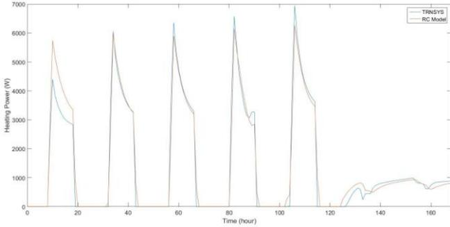
Fig. 4. Heating load for RC model comparing to TRNSYS
