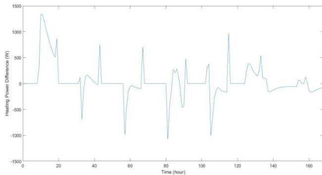
Fig. 6. Heating load error for RC model comparing to TRNSYS
